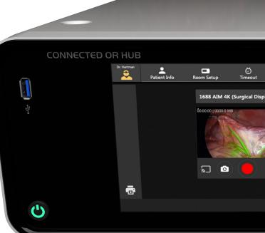
Secure by design: The Connected OR Hub has been updated with several features that improve network security, such as OS hardening, application whitelisting, network vulnerability scans, write protection, and data encryption.
